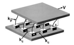
**Figure 6.** Illustration of the two-dimensional sliderblock model. An array of blocks, each with mass m, is pulled across a surface by a driver plate at a constant velocity, V. Each block is coupled to the adjacent blocks with either leaf or coil springs (spring constant  $k_c$ ), and to the driver plate with leaf springs (spring constant  $k_p$ ).
