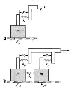
**Figure 5.** Illustration of the slider-block model. (a) A single block of mass m is pulled over a surface by a constant-velocity v driver plate. The plate is connected to the block by a spring with spring constant k. The motion is restricted by a frictional force  $F_s$ . (b) Two blocks with mass m are pulled over a surface. The two masses are connected by a spring with spring constant  $k_c$ . Each mass is connected to the driver plate with spring constant  $k_p$ .
