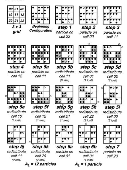
**Figure 1.** Illustration of the sandpile model. A 3 x 3 grid is considered and seven time steps are shown. Model 'avalanches' occur in steps 5 and 6. For the first avalanche, there are ten required redistributions (steps 5b-5k), all nine boxes were 'unstable' at least once, and 12 particles were lost from the grid. In the second avalanche, only one box became unstable, and only one particle was lost from the grid.
